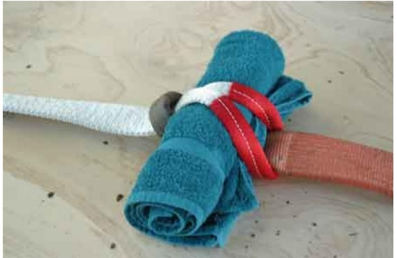
**THIS IS THE RECOMMENDED METHOD, as the towel is not likely to cause too much damage if one of the straps break.**
