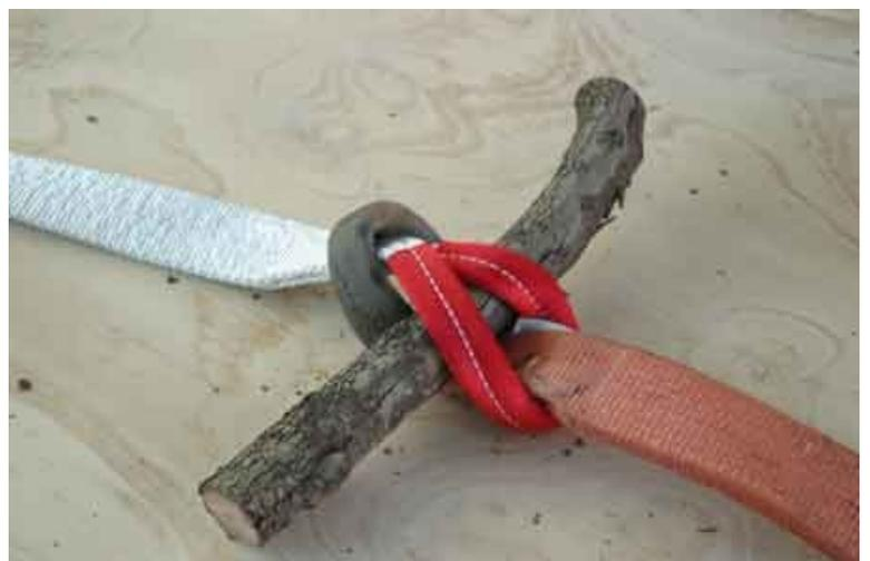
**THIS IS AN ACCEPTABLE METHOD, but the stick will still do damage if one of the straps break.**
