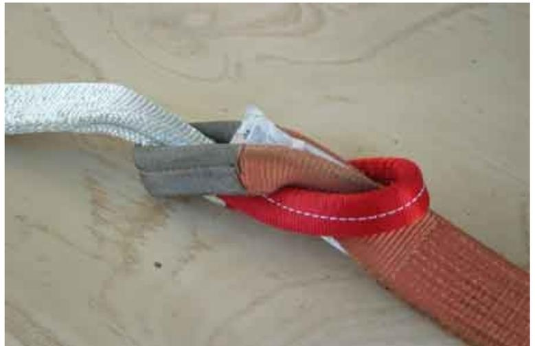
**THIS IS AN ACCEPTABLE METHOD, but the joint will be nearly impossible to undo after use.**
