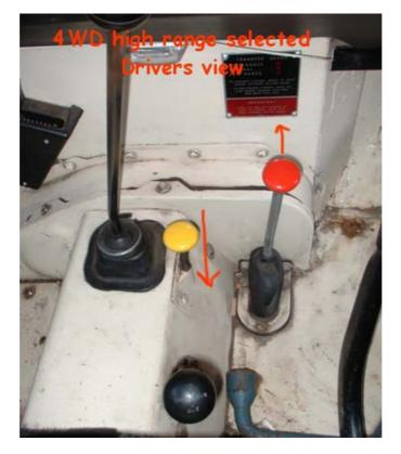
To disengage 4WD whilst in high range, **you must stop**, and then pull back the red lever. As you pull the lever back, the yellow knob will pop back up into its original position. Then push the red lever fully forward again.
