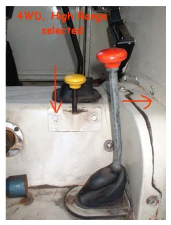
This means that you are now in 4WD, using the normal range of gears as if you were driving normally on the road. You may press down the yellow lever whilst moving, and without depressing the clutch, if necessary. (As long as the free wheeling hubs are engaged, if you have them fitted) The next photo shows the view of the levers from the drivers' seat.
