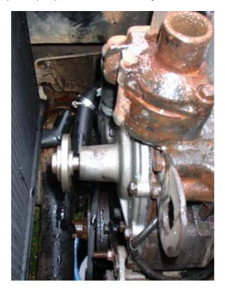
Undo the jubilee clips holding the bypass hose to the pump body and thermostat housing, and then start to remove the bolts holding the pump in position. Military water pumps have 7 bolts, and civilian ones have 9.
