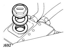
On V8 models, as well as removing the reservoir cap, carefully unscrew the radiator filler plug (illustrated above), allowing pressure to escape before removing completely.
