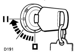
1. With the driver's door closed, insert the key into the starter switch, turn to position 'II' and hold in this position for 5 seconds. Then switch off, and open and close the driver's door.
