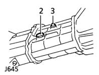
**NOTE:** On some models, to access the main gearbox drain and fill plugs, it will be necessary to remove the rear section of the engine undertray - see 'Engine undertray', earlier in this section.
