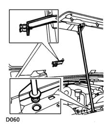
Release the bonnet support stay from the underside of the bonnet and fit the stay in the corresponding hole in the bonnet locking platform.
