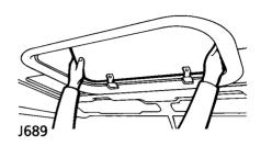
Remove the sunroof by tilting upwards and lifting rearwards to disengage the locating lugs.
