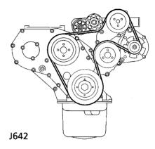
An automatic drive belt tensioner keeps the belt at the correct tension, thereby eliminating the need to manually check the belt deflection.
