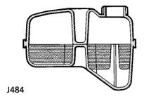
Top-up with a 50% mixture of anti-freeze and water so that the surface of the coolant is level with the seam on the side of the tank. Ensure the cap is tightened fully after top-up is completed.
