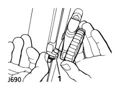
Open the sunroof fully and push the catch (1) rearwards to disengage the hand wheel mechanism.
