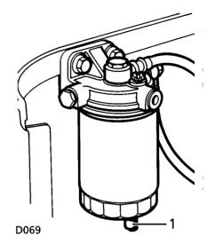
**FUEL FILTER - diesel engines**The filter is located at the front of the engine compartment.
