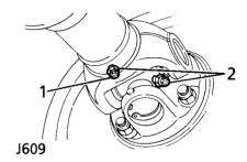
Clean all the grease nipples on the front and rear propshaft universal joints (1).
