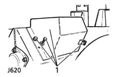
**NOTE:** On 110 models the fuel filter is located behind a protective cover (as illustrated above). To remove the cover, unscrew the three bolts (1).
