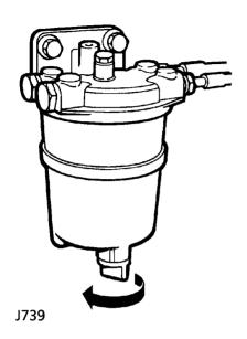
FUEL SEDIMENTER - diesel engines (if fitted)
