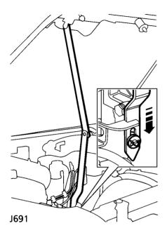
Raise the bonnet until the stay fully extends. Release the bonnet, ensuring that the stay locks into position.
