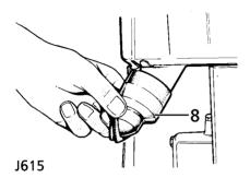
Squeeze open the dump valve (as illustration) and check that the interior is clean. Renew the valve if perished.
