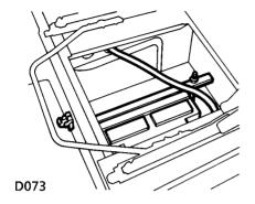
The battery is located underneath the left-hand front seat. Pull up the front of the seat base to release it from its retaining clips and pull it forward. Release the buckle on the front of the battery compartment and slide off the lid.
